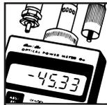
2 Plug your optical connector into the KI screw-on-adaptor.
