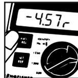
4 To display a relative measurement, push dB/dBm.
