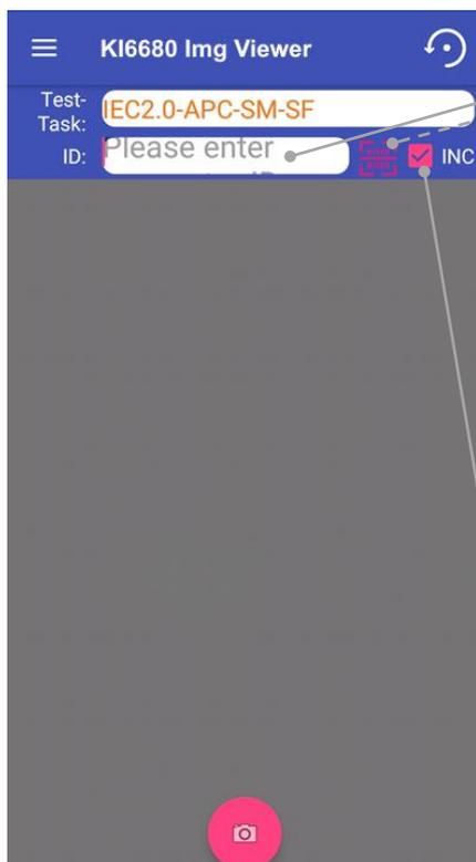
❶ Manually enter text, number, or a combination of text & number in the *ID* field e.g. the ID of the optical fiber.
