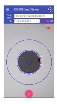
Depending on their sizes, the detected debris/damages are highlighted in red (reject) and/or, yellow (accept) in the different zones (core, cladding, contact) of the optical fiber. These zones are defined by the blue circles.
