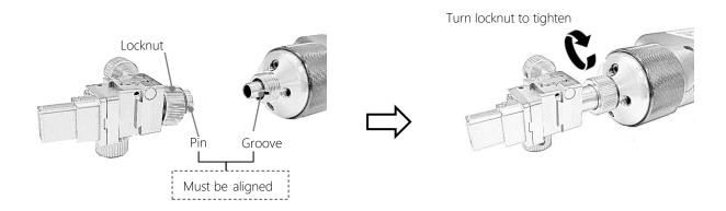
Note: MPO inspection adaptor comes with a PC and an APC tips which are interchangeable by loosening / tightening 2 crews as shown below,
