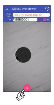
To start analysis, tab on the round camera symbol on software or press the physical button on instrument (see below).
