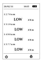
The instrument is now ready for measurements. Power levels of the respective wavelengths in live fibers will be displayed automatically when appropriately connected at OLN & OLT ports.
